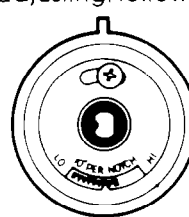
3. To lower the temperature, move black part of knob closer to LO. Each notch equals about 10° F (5° C).
